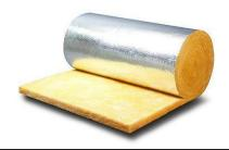
Glass wool is an insulating material made from glass fiber arranged using a binder into a texture similar to wool. The process traps many small pockets of air between the glass and these small air pockets result in high thermal insulation properties.
